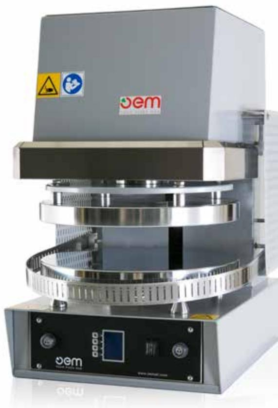
After lifting the plexiglass protection, the plates separate and you can remove the disc. You can now prepare the topping or stack in piles.
